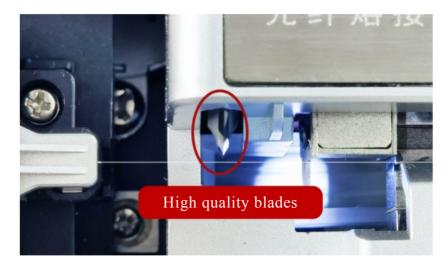
After optical fiber is placed, the cover closed and automatically cut
