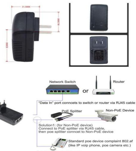
Solution2:(for poe device): Connect to the poe device directly via RJ45 cable
