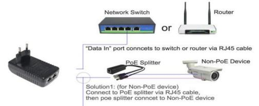
Solution2:(for poe device): Connect to the poe device directly via RJ45 cable
